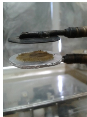
Fig. 1: P25-TiO 2 powder after hydrogenation at \Delta t=40 min plasma exposure time and temperature T=350 °C.
