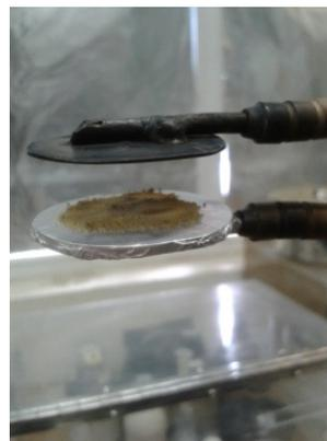
**Fig. 1:** P25-TiO<sub>2</sub> powder after hydrogenation at  $\Delta t=40$  min plasma exposure time and temperature  $T=350$  °C.
