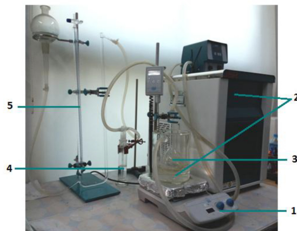
Fig. 1 The experimental setup for catalytic activity tests: 1. Magnetic stirrer 2. Temperature regulated water bath 3. Reactor 4. Washing bottle 5. Gas burette.
